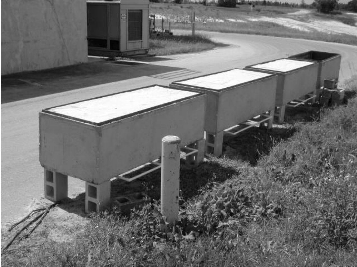
Figure 3.3 Leaching Vaults in Field Loaded with Wood/Tire Ash
