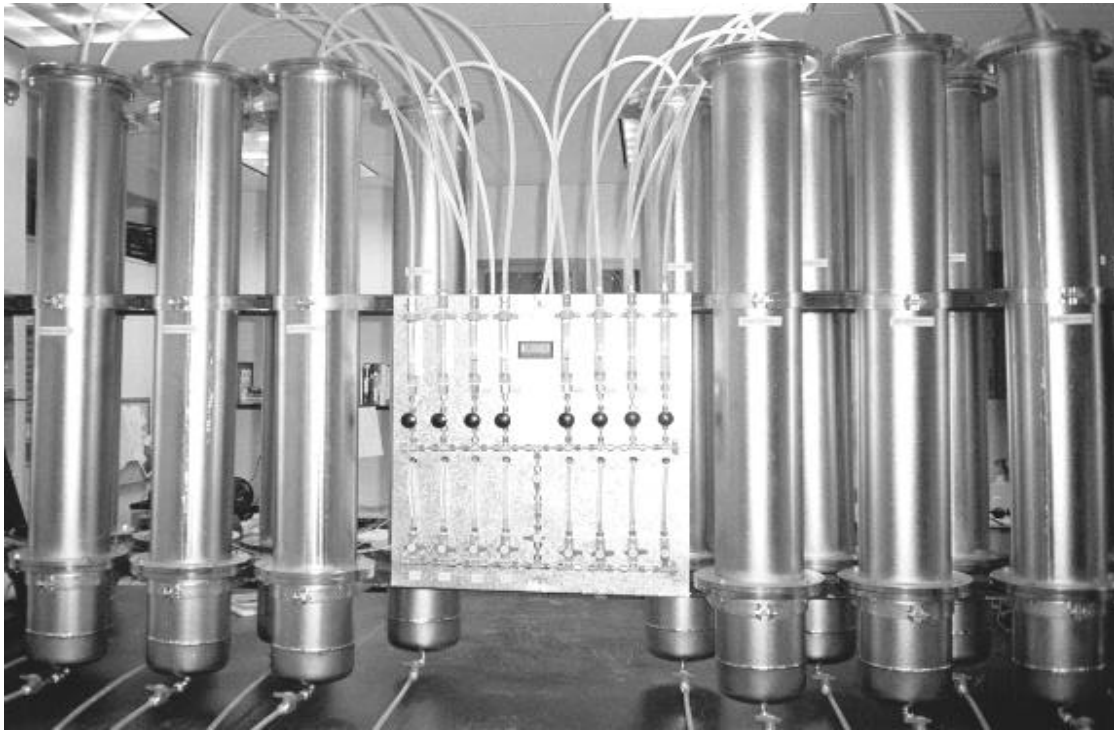
Figure 3.2 Stainless steel column setup
